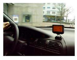
Designed for automobile applications, **E-LOOK** can be mounted on the dashboard or upside down as a ceiling mounted display. A software command permits easy inversion of the screen image.
